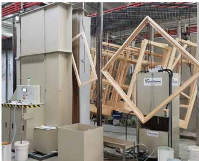
Impregnazione con Flow coating Mod. Polismall Five Impregnation with Flow coating Polismall Five
